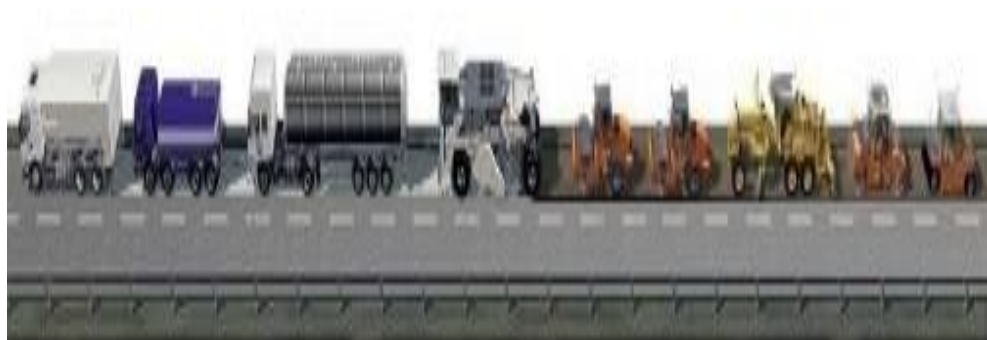
Fig. 3. Echipament single pass tren [4]
